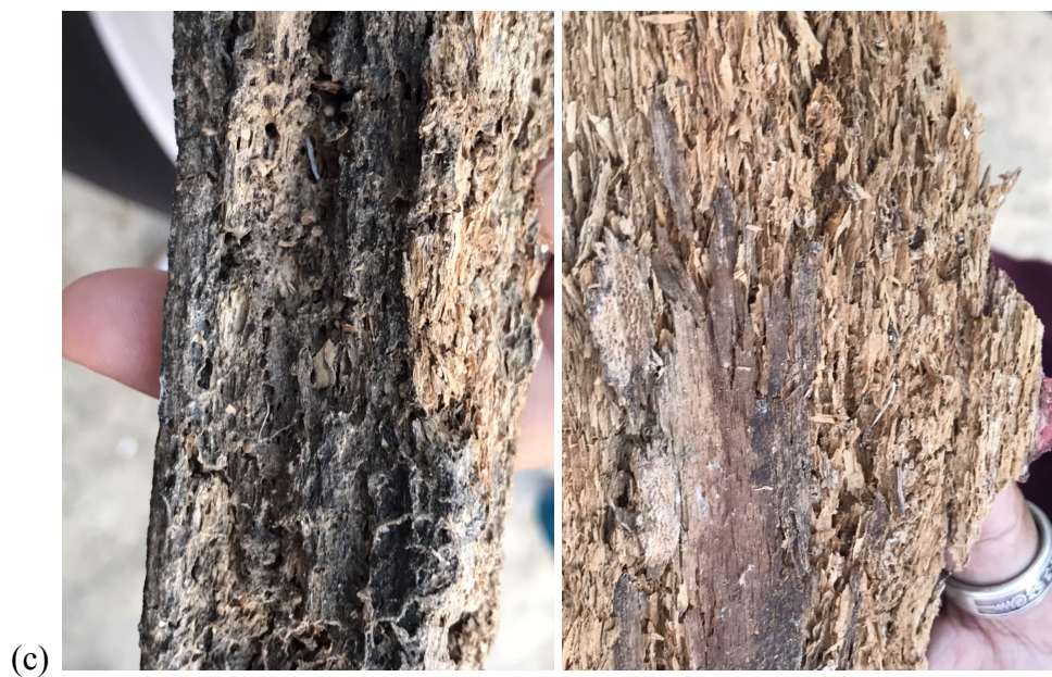
Figure 9: Pieces of the canopy with mold growth, causing them to decay (Location: Zone B). (a) Small holes can be seen between the gaps in the wood panels. (b) Detached sections of
